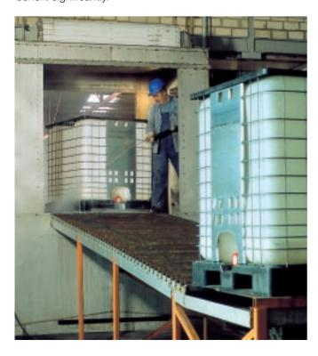
The MAUSER Repaltainer has a modular design, all components are easily removable without deformations or damage to the container. This eases the exchange of parts with new components during the reconditioning process.
