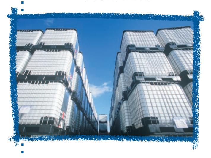
The Composite IBC designed for maximum possible safety and multi-trip use. UN-approved, fully drainable and reconditionable. Available in various types.
